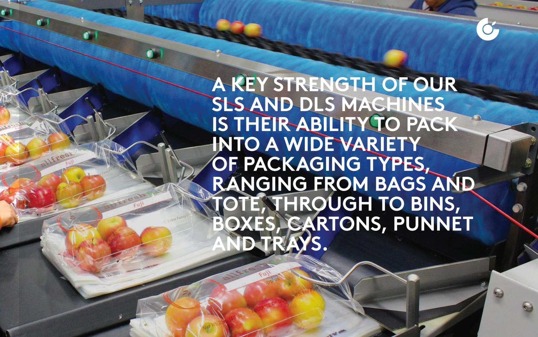
**A KEY STRENGTH OF OUR SLS AND DLS MACHINES IS THEIR ABILITY TO PACK INTO A WIDE VARIETY OF PACKAGING TYPES, RANGING FROM BAGS AND TOTE, THROUGH TO BINS, BOXES, CARTONS, PUNNET AND TRAYS.**
