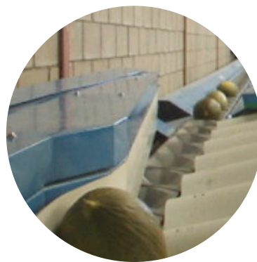
Motorized undulated belt conveyor to ensure a good fruit singulation.
