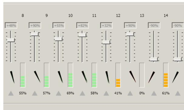
The Compac Dynamic Lane Balancing interface maintains an even flow of cherries across all lanes for maximum efficiency. The system also lets operators monitor the real-time status of the system and alerts them to potential problems.
