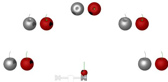
The unique Compac 5 view system analyzes more of the cherry's surface. It also removes false positives which can be caused by the cherry's stem being classified as a defect.
